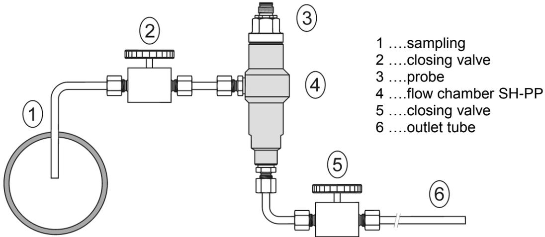
**sampling (1)** - end of the tube placed in the centre of pressure pipelines (distribution of moisture in the pipe cross-section is not homogeneous). To achieve fast response times to shorten the length of the sample tubes to a minimum (few meters).
