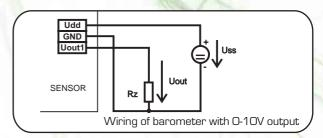
Barometer is directly compatible with sixteen channel Comet data acquisition system MS5D, MS5.
